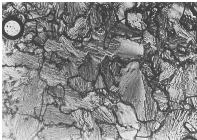
FIGURE 5. Observation of novel optically-observable edge-dislocations in a NOBA LC layer 26 microns thick, U = 200 V, f = 20 kHz
